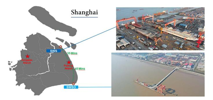
The **SWS yard** spans 361 acres in the Yangtze River estuary with a quayside measuring 1.73km in length and two dry docks. No.1 Dry Dock has two 600-ton gantry cranes tons, and No.2 Dry Dock has two cranes that can lift a respective 800 tons and 600 tons.
