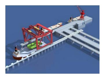
A dedicated float barge is available for modules heavier than 1,200 tons or with unique proportions. The Ro-Ro method will be adopted by SPMTs.
